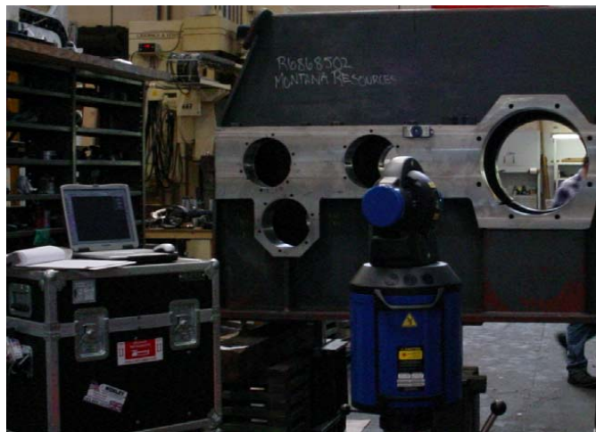
Laser Tracker Measuring Gearbox Bores
