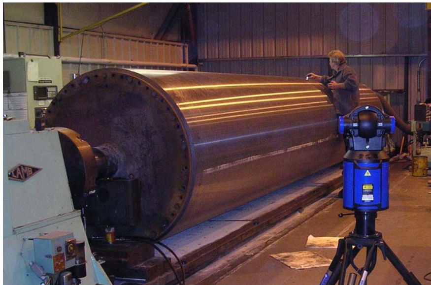
Checking hole drilling positions on a paper mill roll with a Faro Laser Tracker
