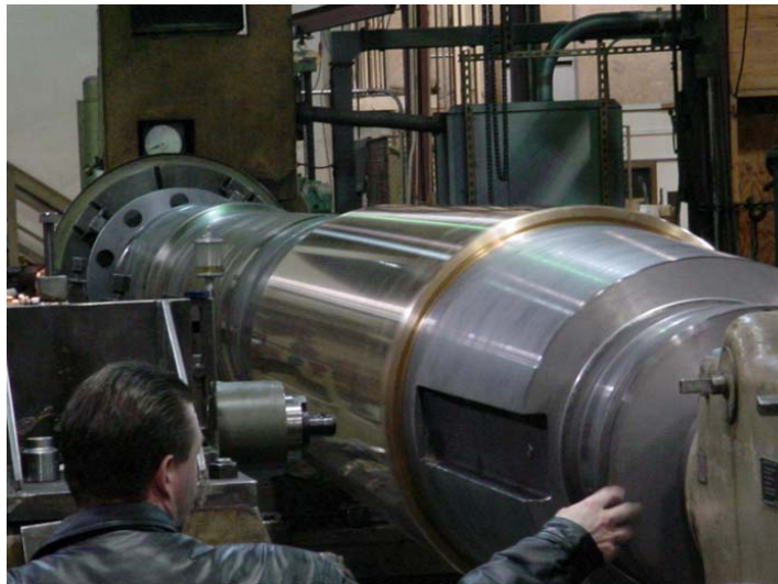
Keyway with milling head in position for machining
